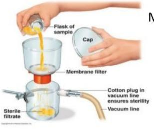
Membrane filters present pores with diameters of µm or nm to effectively remove microorganisms.
